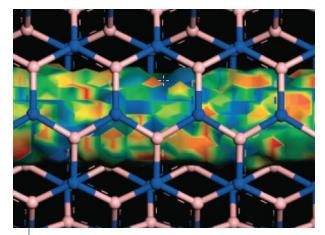
Materials Studio Sorption can be used to study gas storage in nanotubes. The figure represents H2 sorption in a boron-nitride nanotube. Nitrogen atoms are blue and Boron pink. The surface illustrates an isodensity surface of H2 mass density within the nanotube. The surface is colored by the potential energy: red indicates lower energy (tighter binding) and blue higher energy.
